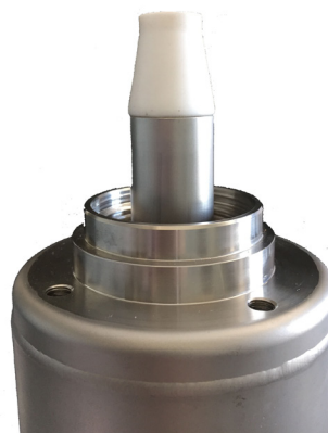
Assembly tool for actuator screw (H338580)
