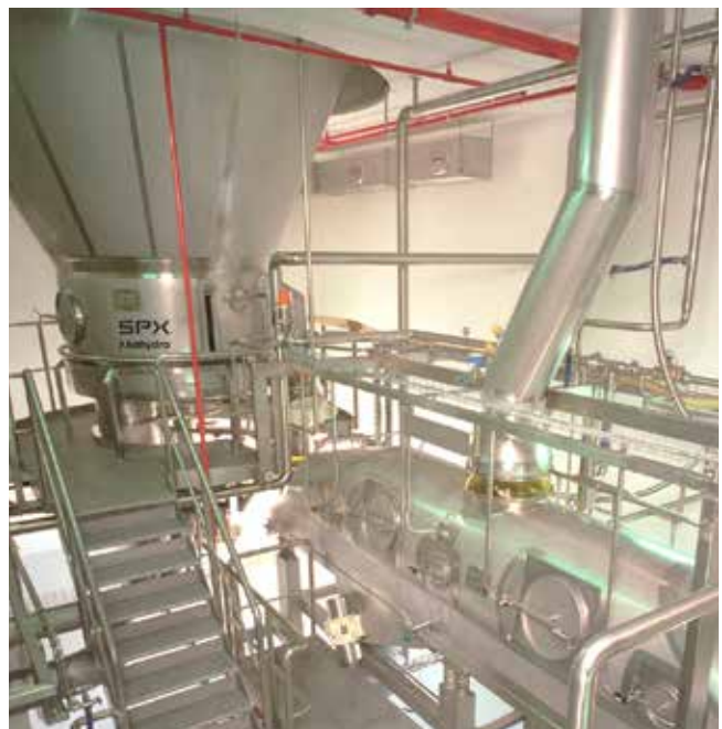
Anhydro spray bed dryer with a fluid bed
