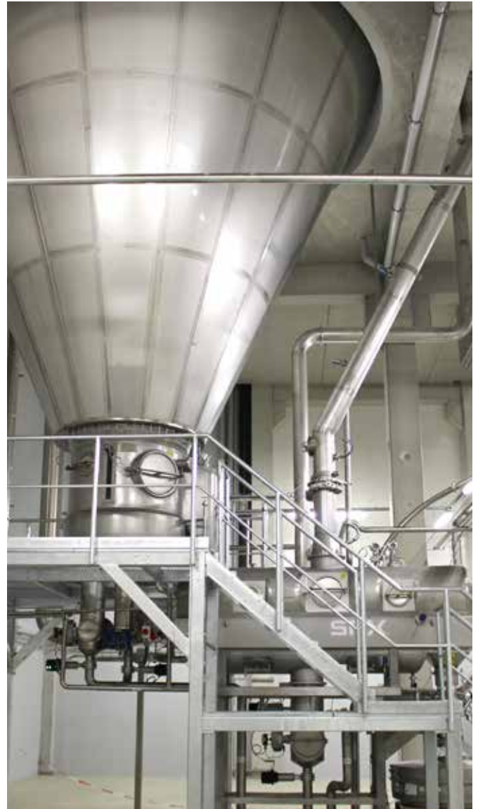
Anhydro spray bed dryer with a fluid bed
