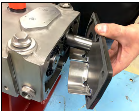
Figure 235 - Install gear case cover
