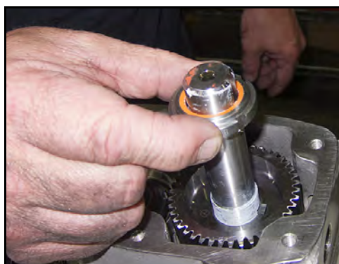
Figure 204 - Install locking nut
