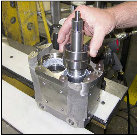
Figure 188 - Place outer race on shaft
