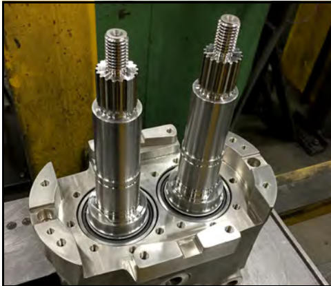
Figure 192 - Shafts seated in gearcase
