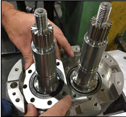
Figure 199 - Install bearing retainer
