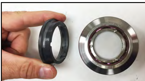
Figure 73 - Lubricate and install seal
