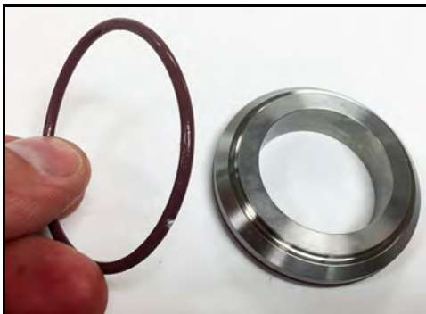
Figure 45 - Remove cap-to-screw O-ring
