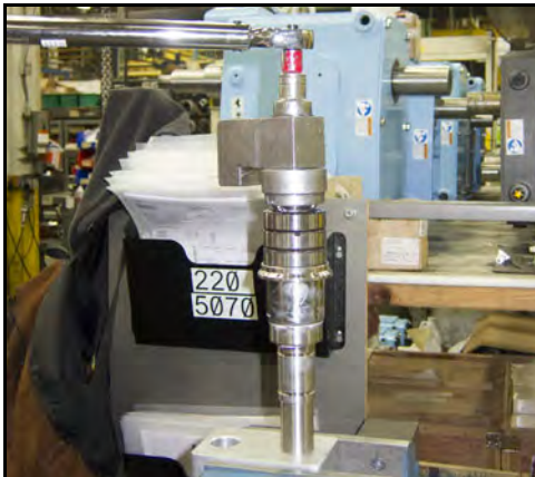
Figure 179 - Torque down locking nut
