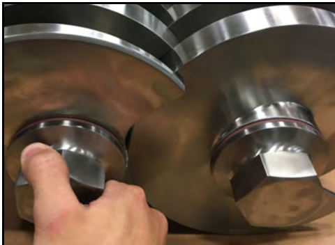
Figure 124 - Install screw nuts
