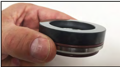
Figure 102 - Seal seat installed on seal cap
