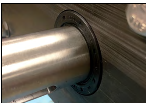
Figure 239 - Oil seal installed
