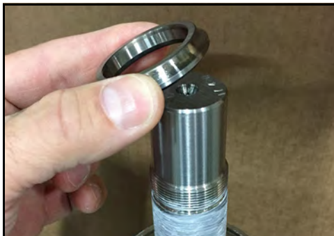
Figure 162 - Place race onto shaft
