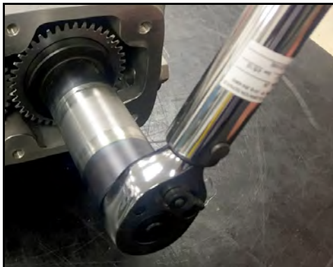
Figure 141 - Loosen locking nut
