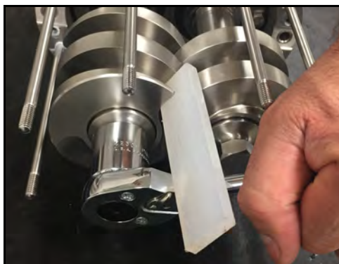
Figure 219 - Tighten screw nut
