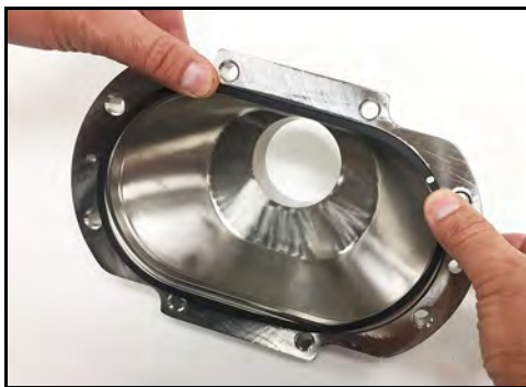
Figure 127 - Install cover gasket
