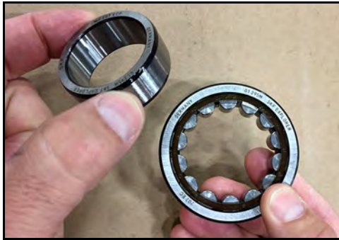
Figure 174 - Remove race from bearing
