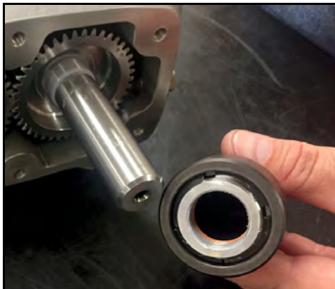
Figure 142 - Remove locking nut and gear
