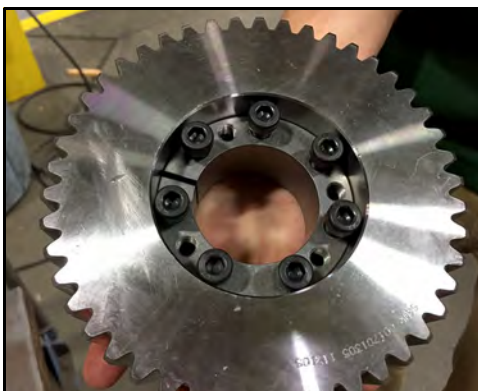
Figure 212 - Place locking assembly into gear
