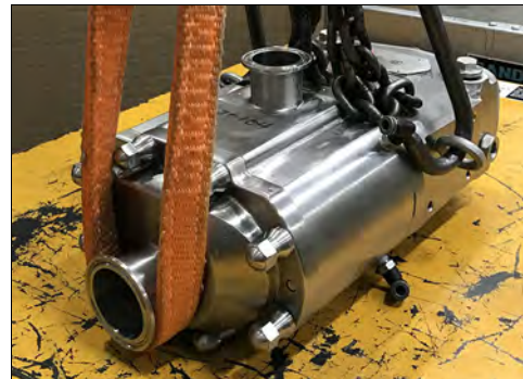
Figure 2 - Lifting location detail - 015, 030-UTS
