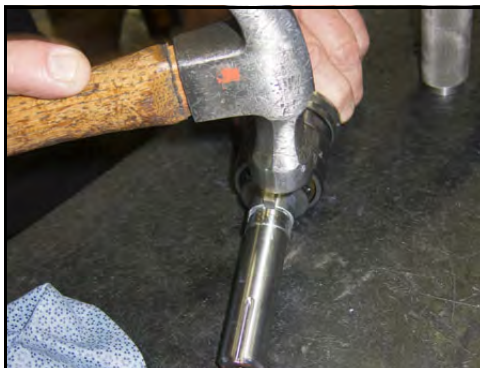
Figure 182 - Tap key into keyway
