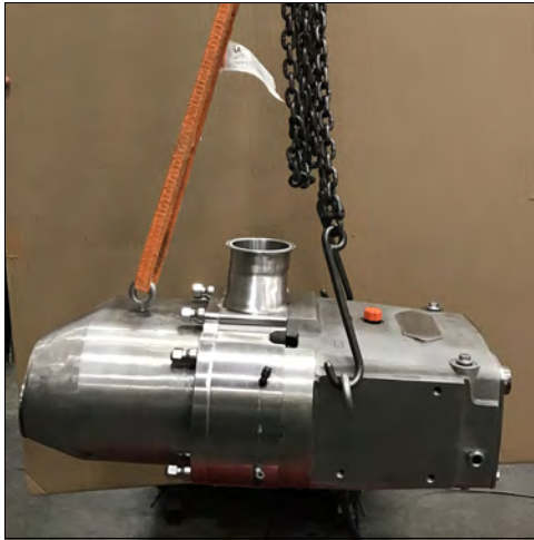
Figure 3 - Lifting location - 130, 220-UTS
