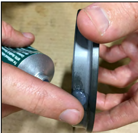
Figure 81 - Lubricate the outer diameter of the seal
