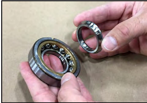
Figure 160 - Remove bottom race
