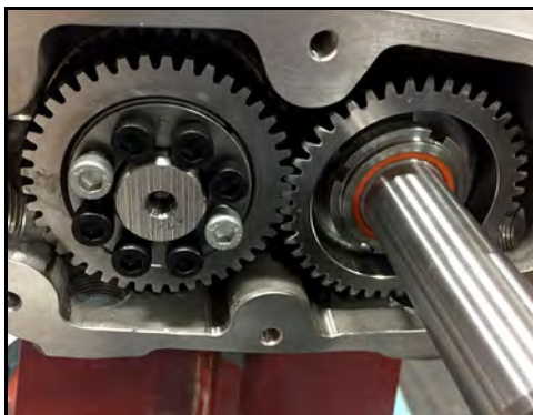
Figure 214 - Align loose gear with drive gear
