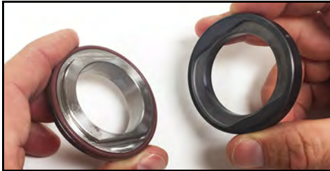
Figure 101 - Line up seal cap and seal seat
