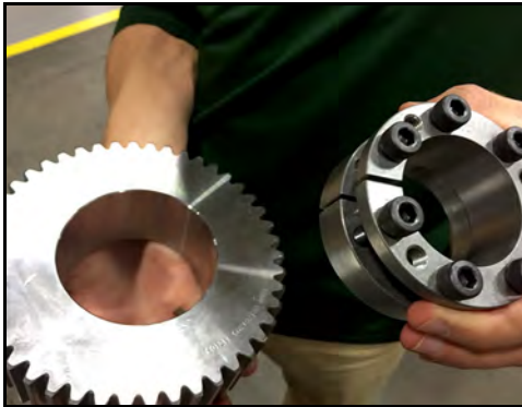
Figure 211 - Assemble locking assembly into gear
