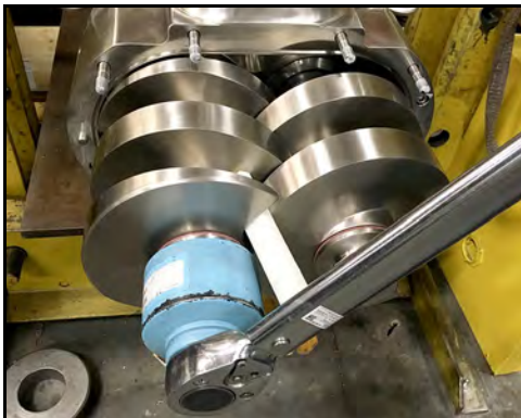
Figure 125 - Torque left screw nut
