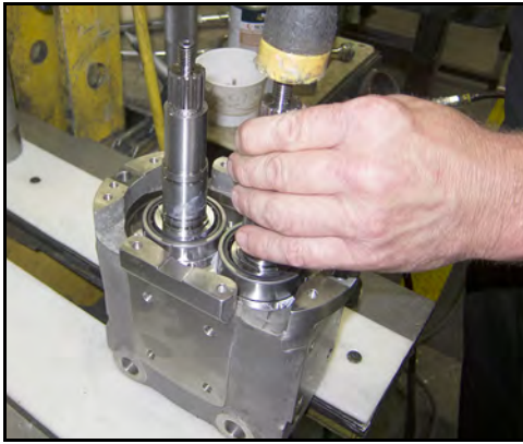
Figure 191 - Tap shafts to center in bores
