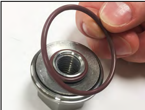
Figure 116 - Install screw nut O-ring
