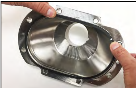
Figure 29 - Remove cover gasket
