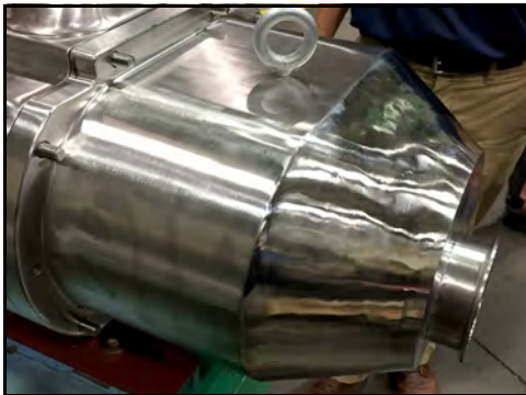
Figure 130 - Seat pump cover against pump body
