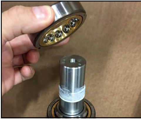
Figure 170 - Place bearing onto race
