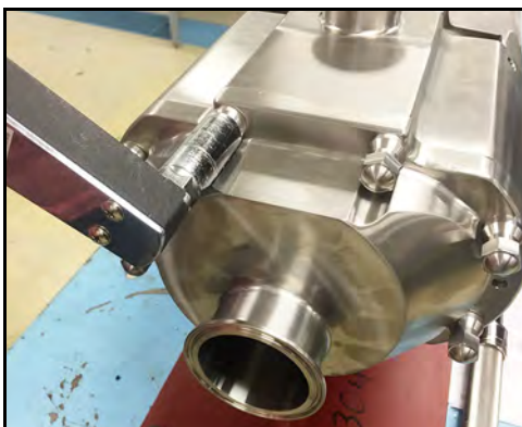
Figure 132 - Torque cover nuts
