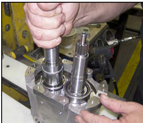
Figure 189 - Place drive shaft in bore
