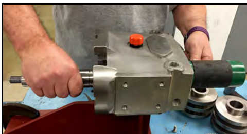
Figure 147 - Tap short shaft out of gear case
