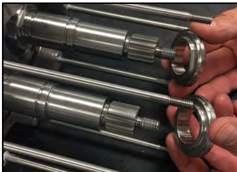
Figure 215 - Install seal caps
