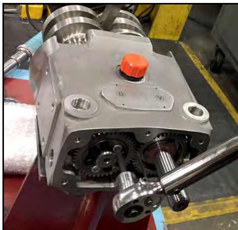
Figure 227 - Torque locking assembly bolts
