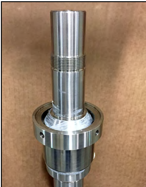
Figure 158 - Bearing spacer installed
