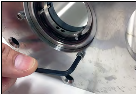
Figure 80 - Install with cap screws
