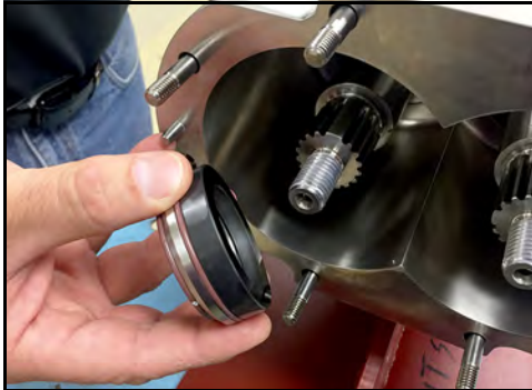
Figure 43 - Remove seal cap assembly
