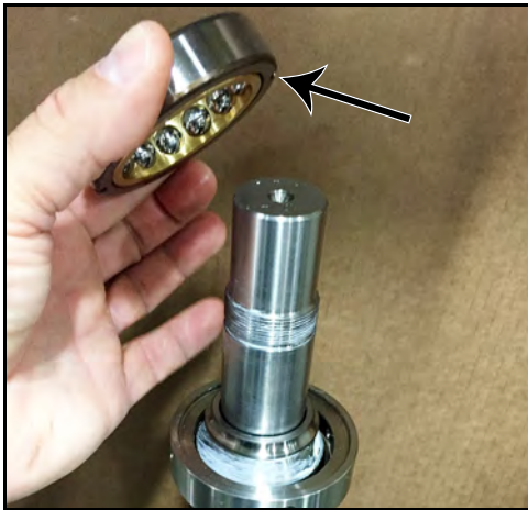
Figure 165 - Place bearing onto race
