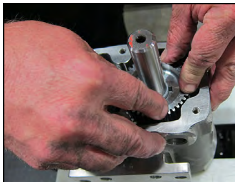
Figure 203 - Install drive gear
