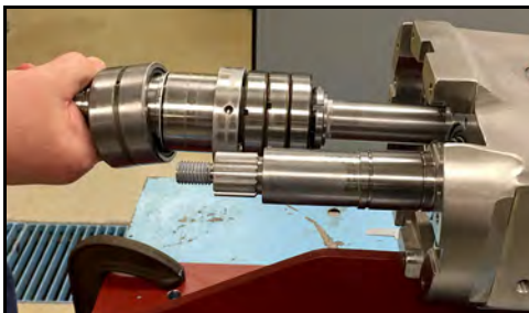
Figure 146 - Pull drive shaft out of gear case
