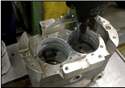
Figure 185 - Spread even layer
