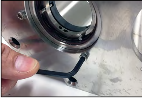
Figure 56 - Remove cap screws
