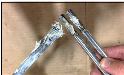
Figure 89 - Apply anti-seize to threads
