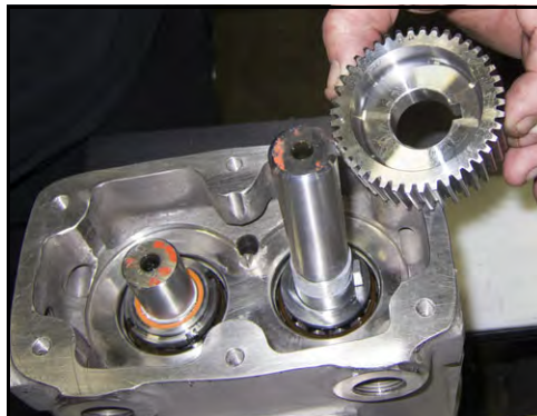
Figure 202 - Install drive gear
