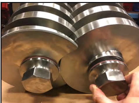
Figure 37 - Remove screw nuts
