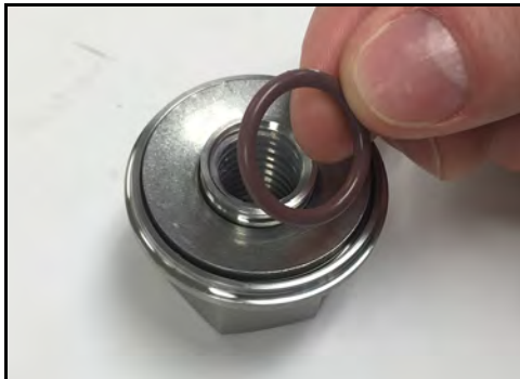
Figure 39 - Remove washer retainer O-ring
