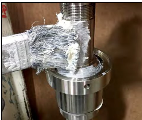
Figure 161 - Apply anti-seize to shaft
