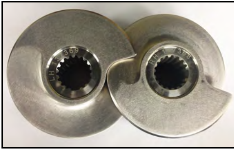
Figure 42 - Screws arranged LH - RH
