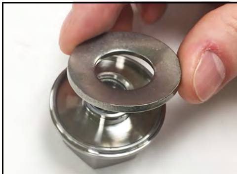
Figure 40 - Install Belleville washer
