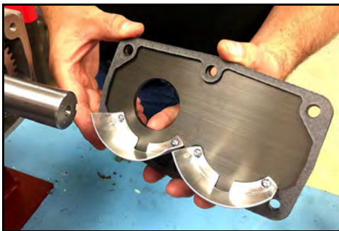
Figure 234 - Place gasket on cover
