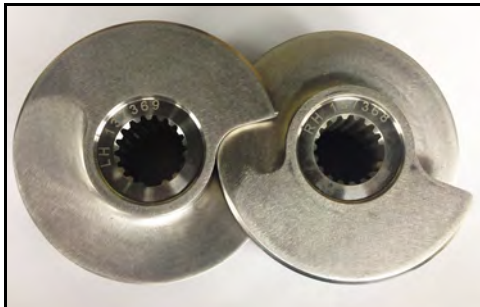
Figure 107 - Arrange screws: LH-RH
