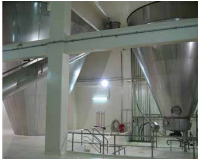
A section of a dairy drying system - a drying chamber cone and a bag filter bottom
