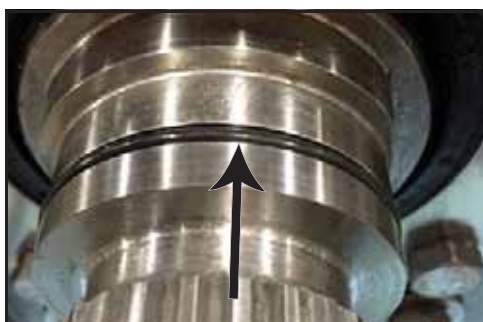
Figur 69 - O-ring for justeringsring
