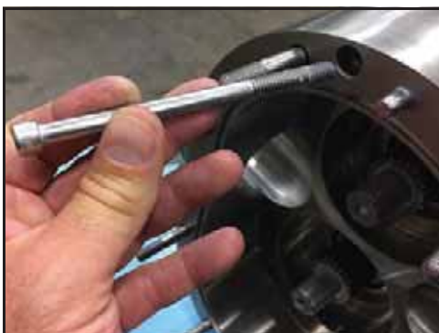
Figur 129 - Installere pumpehusets holdeskruer
