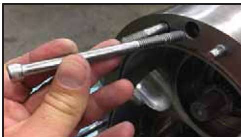
Figur 42 - Demontere pumpehusets holdeskruer
