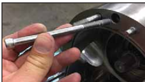
Figur 147 - Demontere pumpehusets holdeskruer
