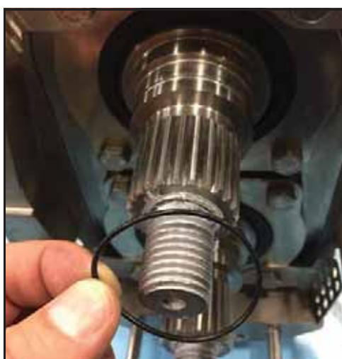
Figura 119 - Instalar o anel O-ring
