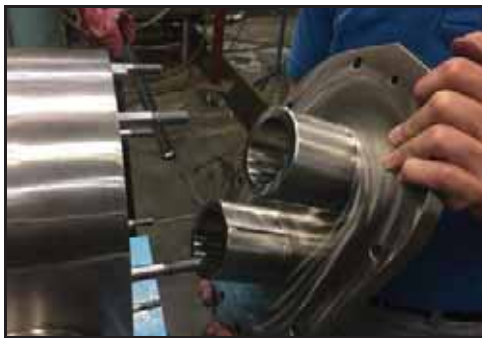
Figura 186 - Instalar a tampa
