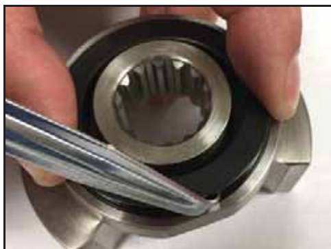
Figura 140 - Pressionar o anel O-ring
