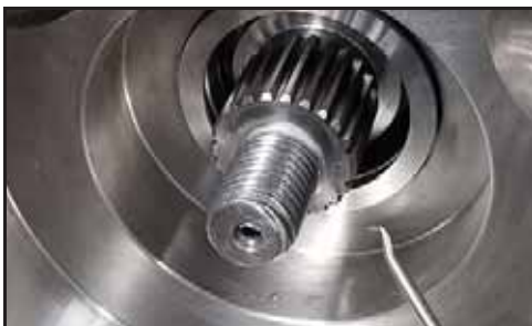
Figura 144 - Remover o anel O-ring
