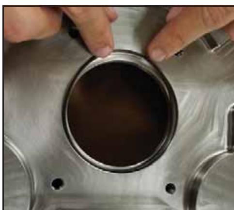
Figura 151 - Remover o anel O-ring
