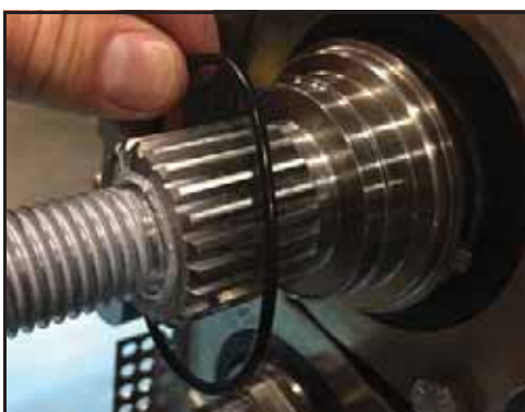
Figura 123 - Instalar o anel O-ring
