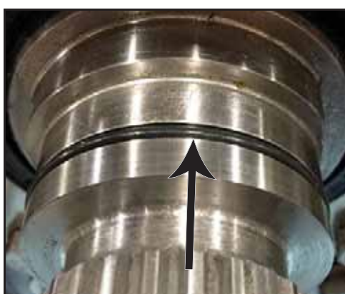
Figura 120 - Anel O-ring instalado
