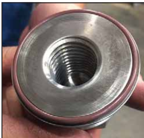
Figura 180 - Anel O-ring instalado
