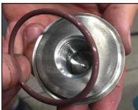
Figura 36 - Remover o anel O-ring
