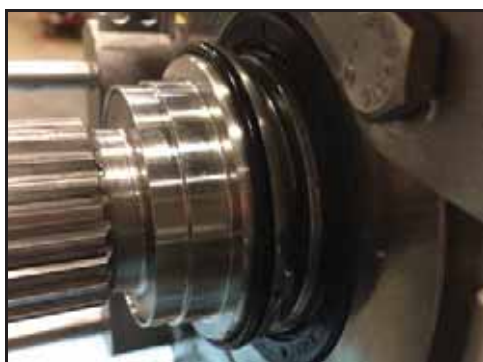
Figura 104 - Anel O-ring instalado
