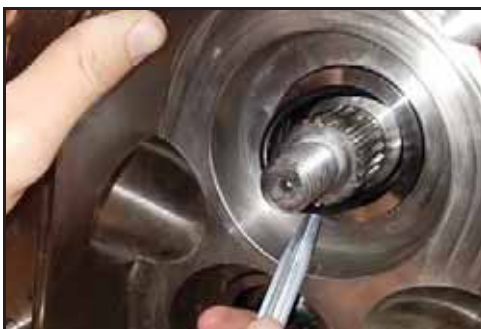
Figura 143 - Remover o anel O-ring
