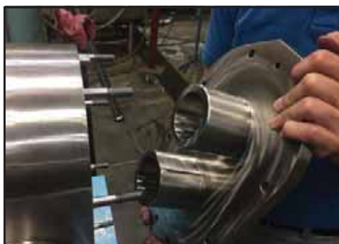
Figura 33 - Remover a tampa
