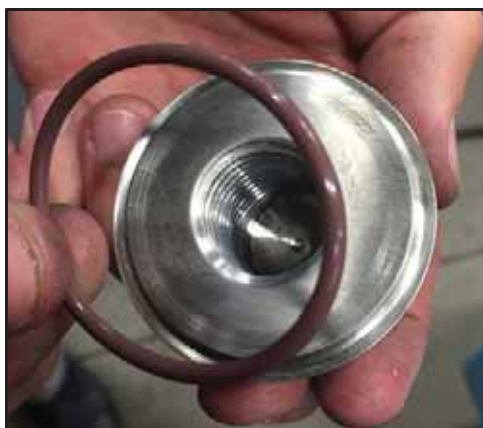
Figura 179 - Instalar o anel O-ring
