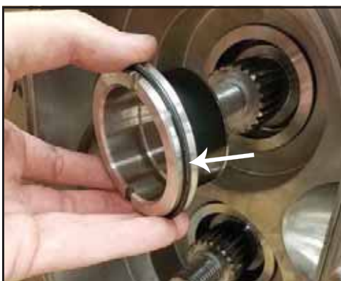
Figura 142 - Remover a luva, anel O-ring
