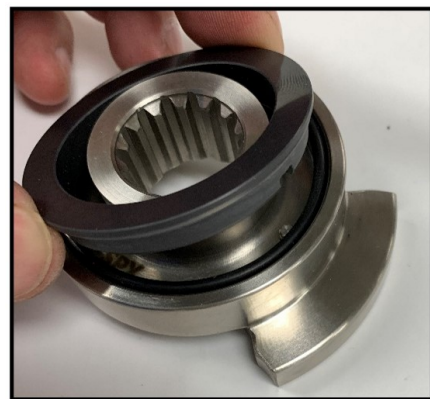
Figure 115 Install rotary seal
