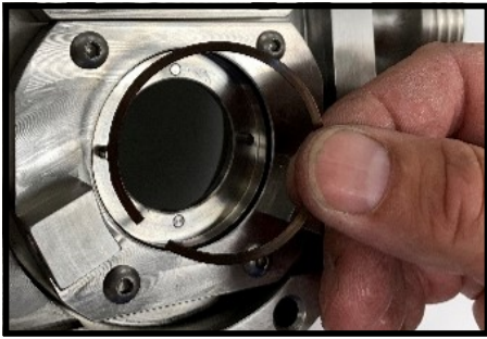
Figure 98 Install stationary sela wave spring
