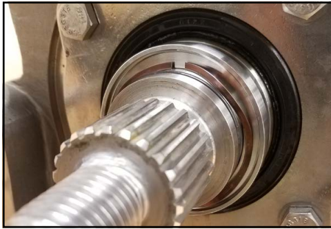
Figure 242 - Install wave spring
