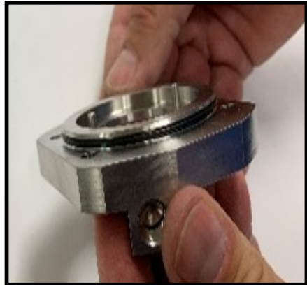
Figure 92 Install the seal housing O-ring
