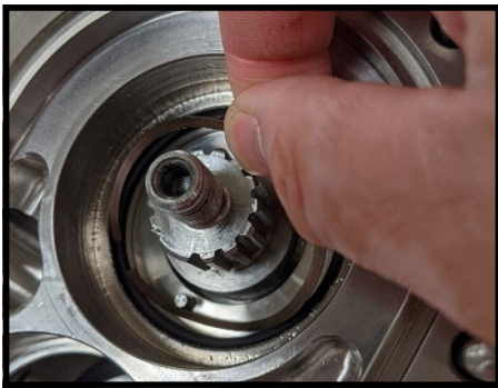
Figure 111 Install stationary wave spring
