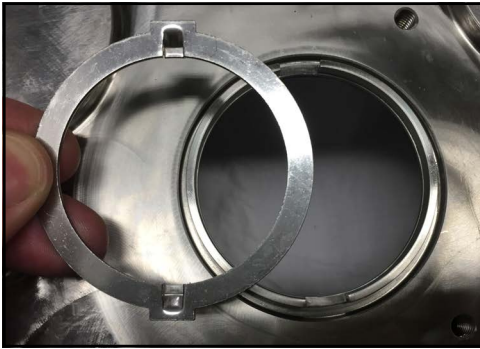
Figure 131 - Install drive ring
