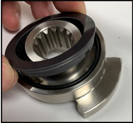
Figure 52 Remove rotary seal
