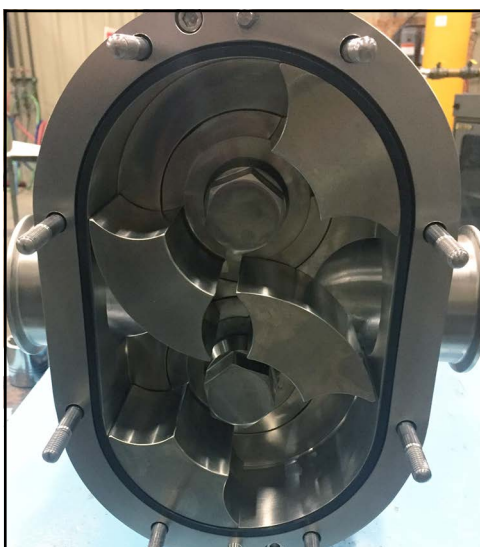
Figure 263 - Cover gasket installed
