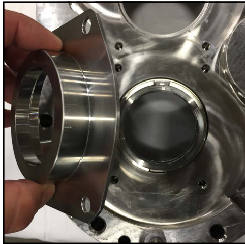
Figure 135 - Install seal housing
