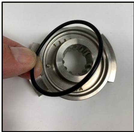
Figure 114 Install seal O-ring
