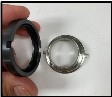
Figure 82 Remove flush side rotary seal and O-ring
