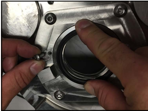
Figure 174 - Install seal retaining bolts
