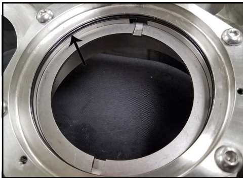
Figure 192 - Seal O-ring location
