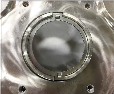
Figure 132 - drive ring installed (134-U3 and smaller)
