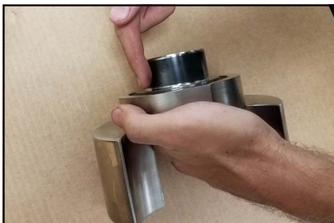
Figure 252 - Lubricate seal sleeve
