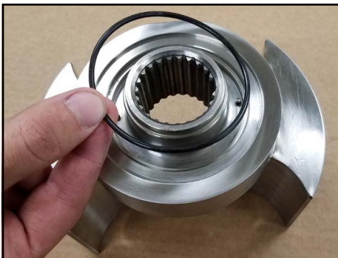
Figure 247 - Install sleeve front O-ring
