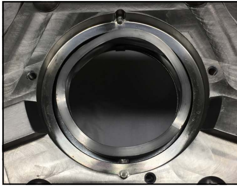
Figure 171 - Wave spring installed
