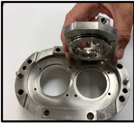
Figure 94 Install seal housing
