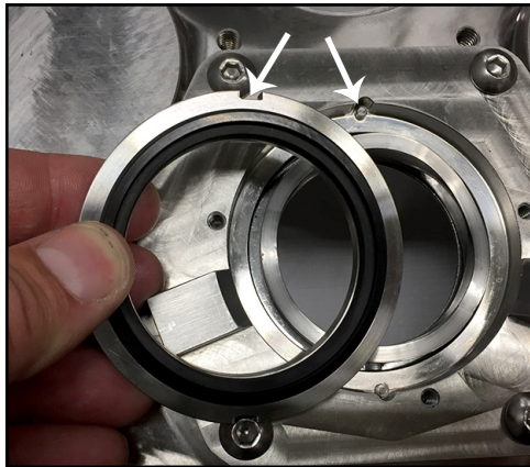
Figure 172 - Install flush-side stationary seal
