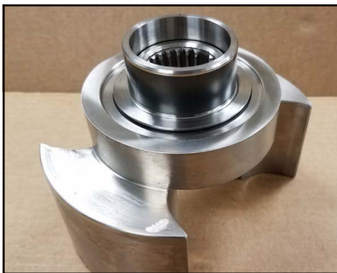
Figure 251 - Seal sleeve installed
