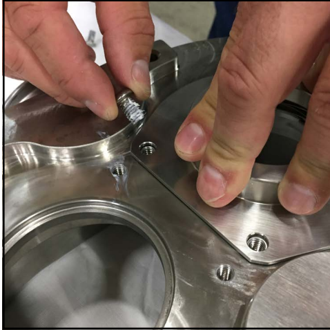
Figure 122 - Remove seal housing bolts
