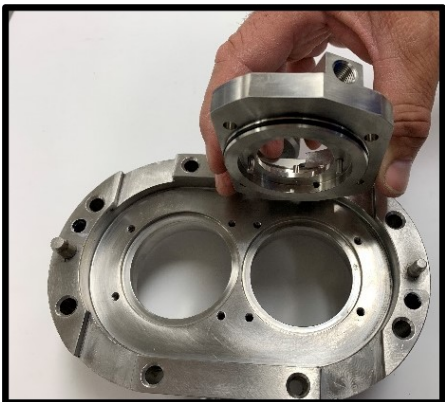
Figure 89 Remove seal housing
