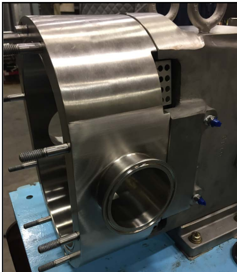
Figure 244 - Pump body installed
