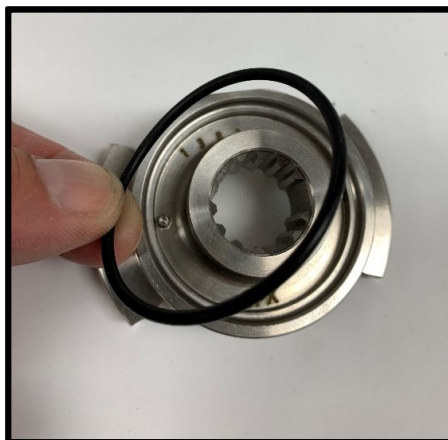
Figure 75 Remove seal O-ring
