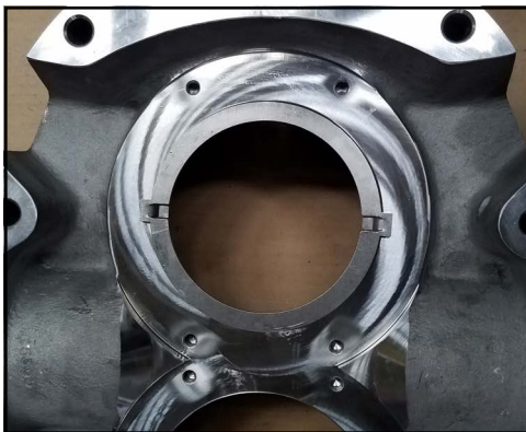
Figure 186 - Drive ring installed
