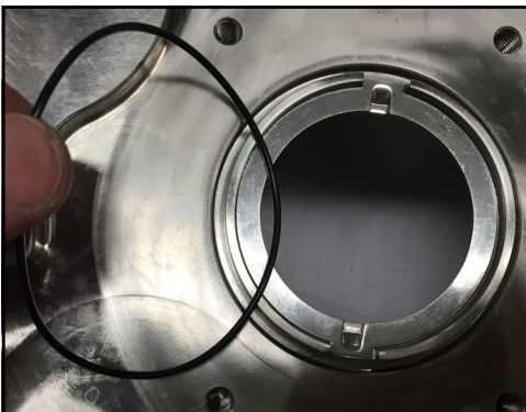
Figure 154 - Remove seal housing O-ring
