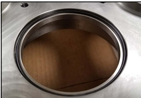
Figure 233 - Seal housing O-ring installed
