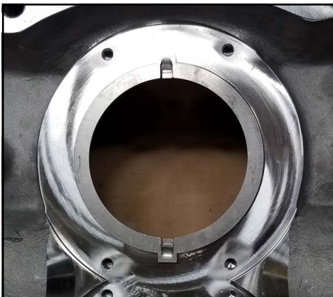
Figure 139 - Drive ring installed
