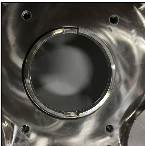
Figure 160 - Shaft ring installed
