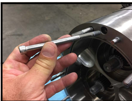
Figure 57 Remove body retaining screws
