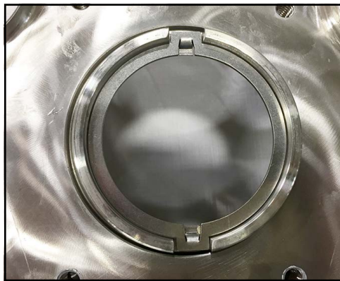
Figure 162 - Drive ring installed
