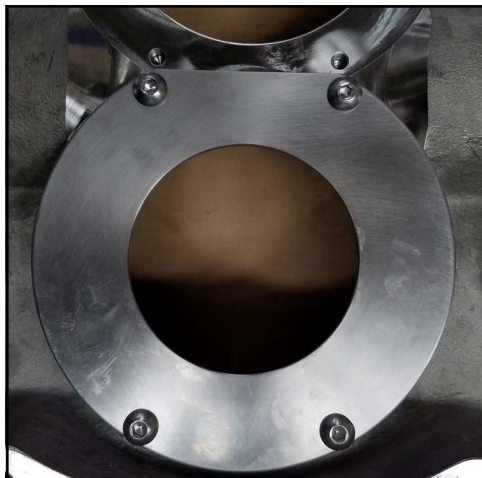
Figure 143 - Seal housing installed
