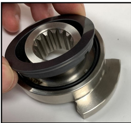
Figure 51 Install rotary seal
