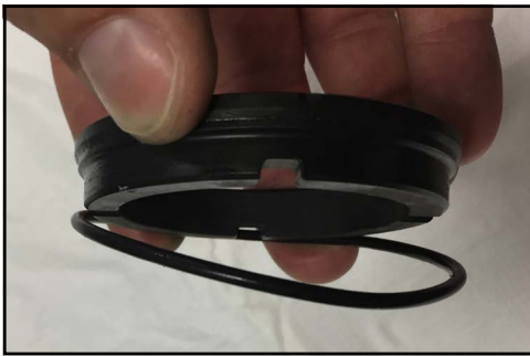
Figure 119 - Remove stationary seal O-ring
