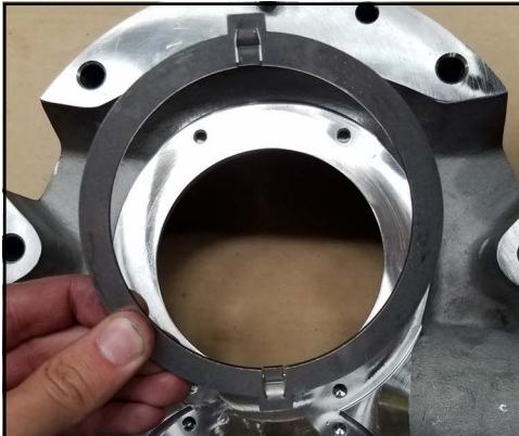
Figure 138 - Install drive ring
