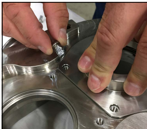
Figure 136 - Install seal housing bolts
