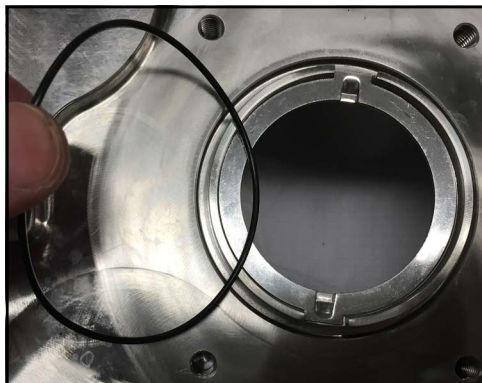
Figure 163 - Install seal housing O-ring
