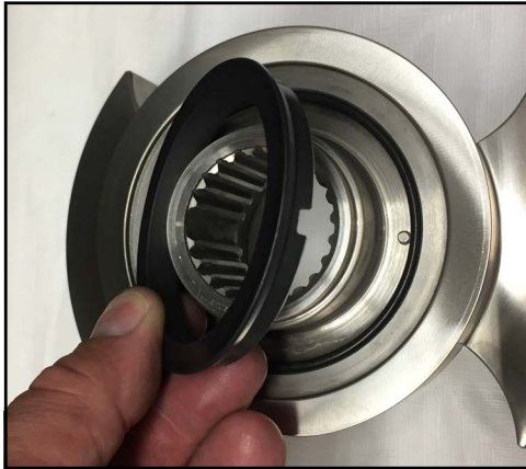
Figure 116 - Remove rotary seal
