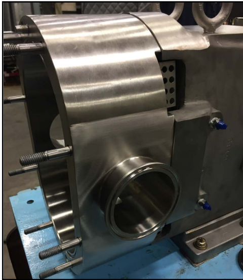
Figure 66 - Pump body installed
