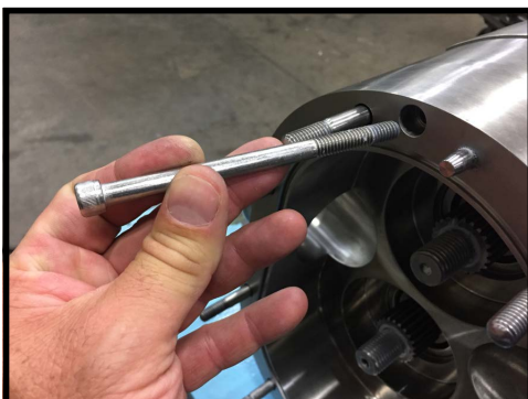
Figure 109 - Install body retaining screws
