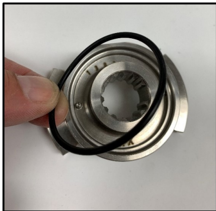
Figure 72 Install seal O-ring
