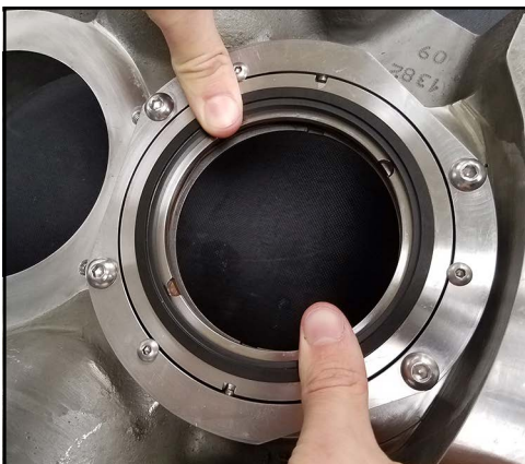
Figure 196 - Apply finger pressure
