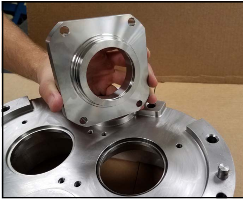
Figure 234 - Line up bolt holes
