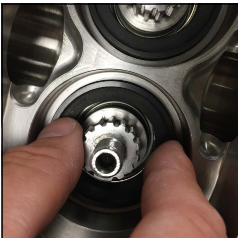
Figure 211 - Push on stationary seal
