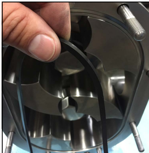
Figure 37 - Remove cover gasket
