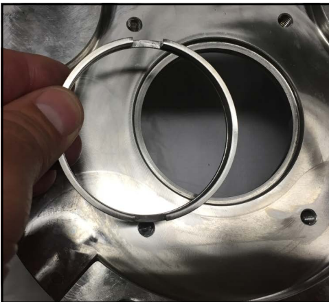
Figure 127 - Remove shaft ring
