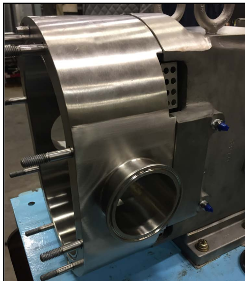
Figure 206 - Pump body installed
