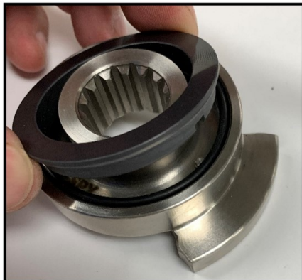
Figure 74 Remove rotary seal
