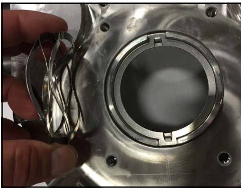
Figure 133 - Install wave spring
