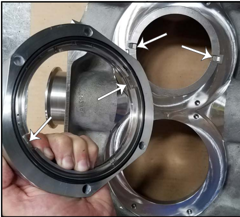
Figure 188 - Seal housing O-ring installed
