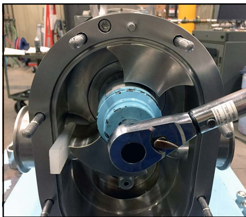
Figure 260 - Torque rotor nut
