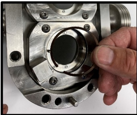
Figure 86 Remove stationary seal wave spring
