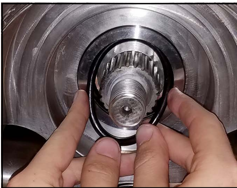
Figure 246 - Install seal O-ring
