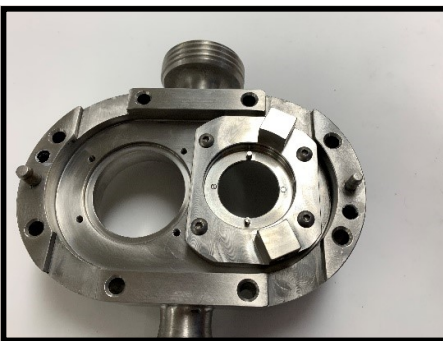
Figure 96 Seal housing installed
