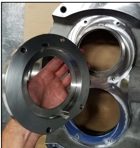
Figure 124 - Remove seal housing
