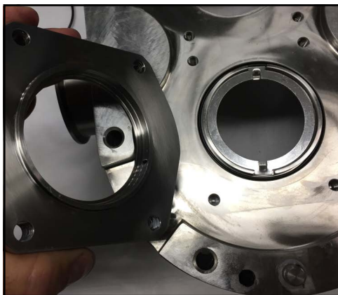
Figure 165 - Install seal housing
