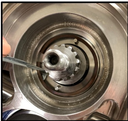
Figure 78 Remove stationary seal wave spring
