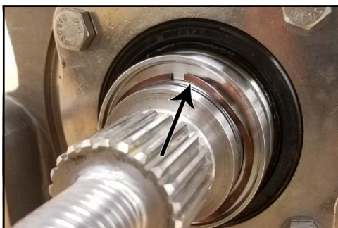
Figure 230 - Remove wave spring
