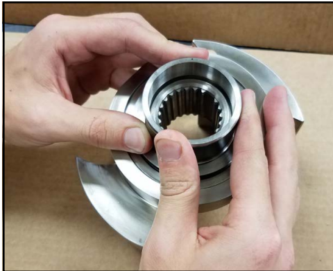
Figure 250 - Press sleeve into place
