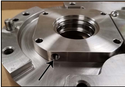
Figure 235 - Flush hole location
