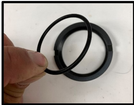
Figure 103 Install flush side rotary O-ring
