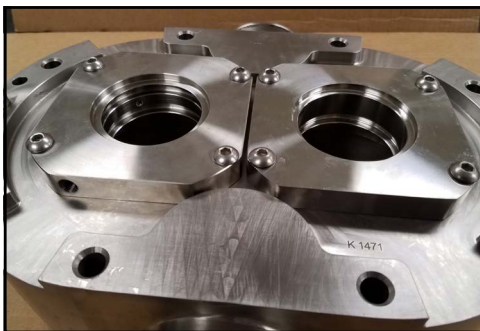
Figure 237 - Seal housings installed
