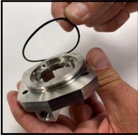
Figure 90 Remove seal housing O-ring
