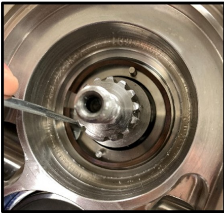
Figure 45 Remove stationary seal wave spring
