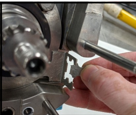
Figure 106 Break tab off finger guard
