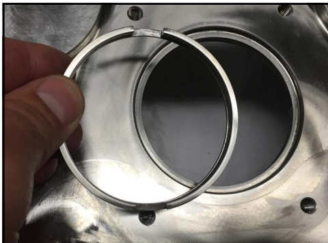
Figure 157 - Remove shaft ring
