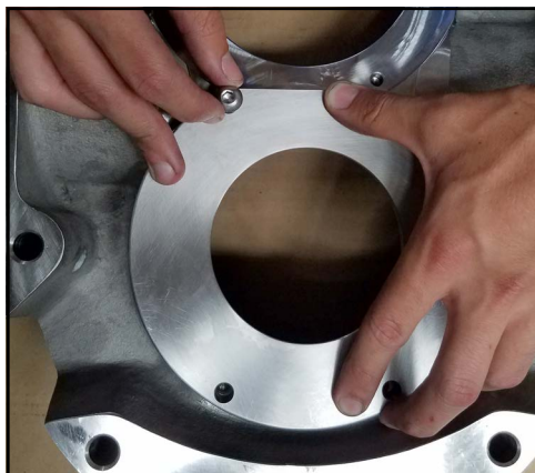
Figure 142 - Install seal housing bolts
