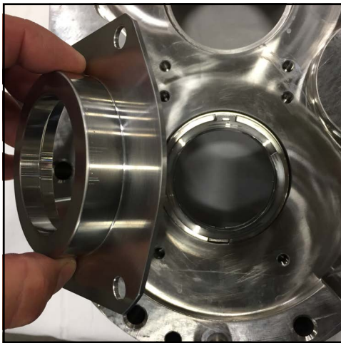
Figure 123 - Remove seal housing
