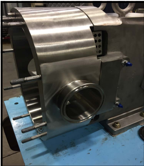
Figure 108 - Pump body installed
