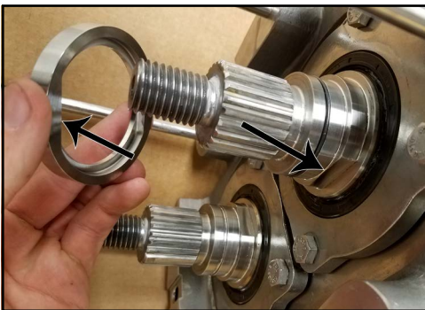
Figure 240 - Install seal seat
