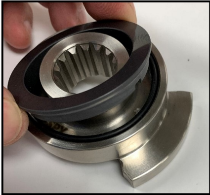
Figure 41 Remove rotary seal
