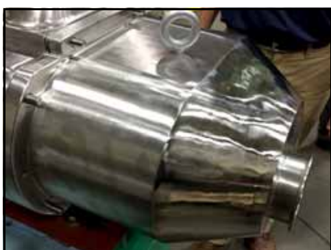
Figur 130 - Still pumpedekselet mot pumpehuset
