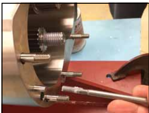
Figur 51 - Demontere pumpehusets holdeskruer
